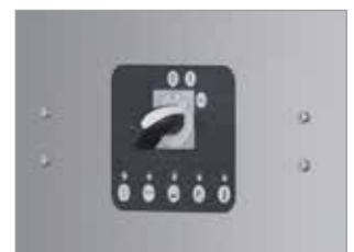
CONTROL PANEL SHOWING: ON/OFF SWITCH, NETWORK INDICATOR LIGHT, FLAME CONTROL LIGHT, WARMING LACK OF ANTISCALE, SERVICE WARNING LIGHT (150 HRS), READY WARNING LIGHT (TEMPERATURE REACHED)
